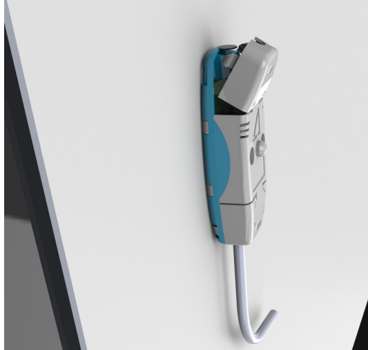
Figure 2: Modern arc light point sensors may be wired in series making the overall installation and wiring faster and more convenient. The most advanced sensors are able to monitor continuously even the photodiode element by integrated light pulse source. The light pulse also feedbacks users on the ready state of the sensor.
