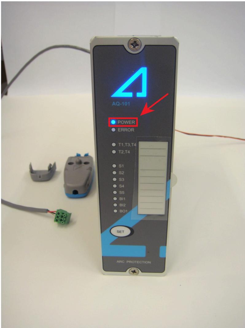
5. Attach the connector back into its slot in the sensor PCB (see the red arrow in the image below; the connector is already in place on the right side).
