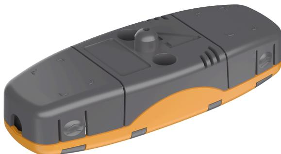
An AQ-02 can only be installed on the compartment wall as not to block pressure detection located next to "the eye". The unit placed on the wall (with the gray side against the wall), and then fixed to the wall with two screws. No external mounting plates are needed regardless of the mounting type; however, mounting brackets can be used if so desired.
