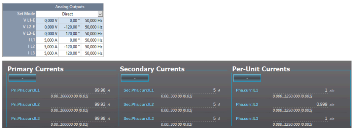
Figure. 5.2.1 - 9. Scalings display (based on the protected object's nominal current).
