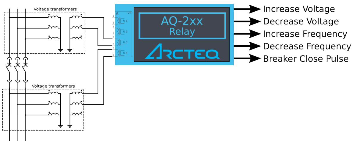
Figure. 5.5.9 - 184. Simplified presentation of synchronizer operation
